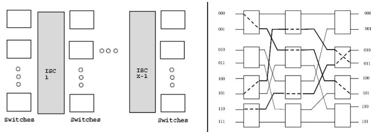
Figure 1: Multistage interconnection network and an example  $8 \times 8$  Shuffle-Exchange network (SEN).
